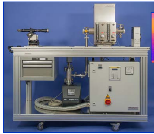
High temperature contact angle measuring system with vacuum or inert gas OCA 25-HTV 1800
