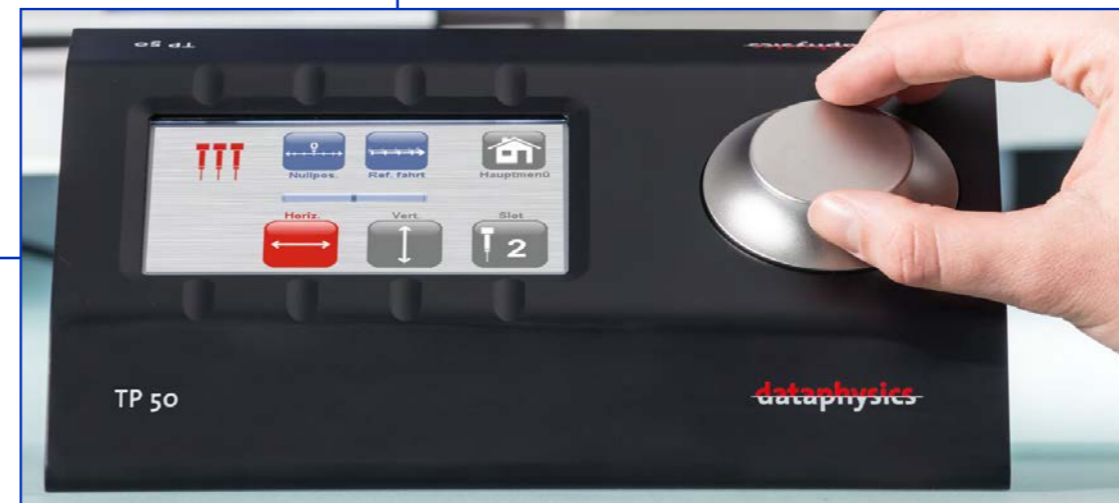
TP 50 control panel with touch screen
