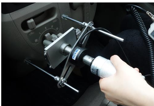
For feeling test of rotary switches on car dashboard
