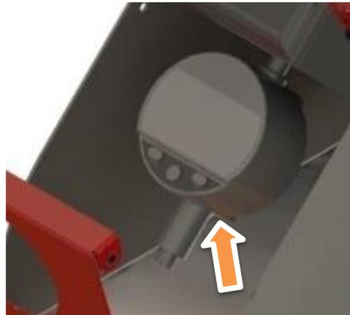
Remember that after changing the battery the device must be calibrated, or set to zero.
