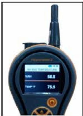
Figure 4: Hygromaster2 as a Hygrometer
