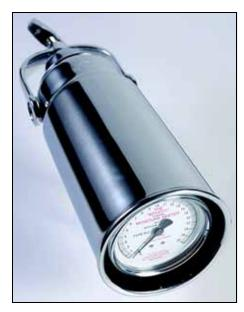
A standard size speedy is shown in the photograph to the left. The moisture test procedure is simple to follow and takes a just few minutes for most materials. However, to ensure accurate and consistent results the procedure should be followed precisely. To test your sample, refer to the photographs below and complete the following steps:
