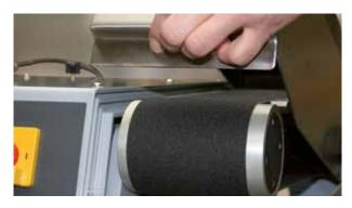
It is possible to use belts with 2 different grain sizes simultaneously.
