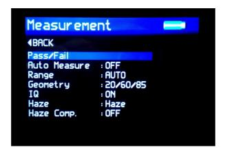
The Measurement Screen is used to configure the instruments measurement parameters to the user's preference. Pressing the Up and Down buttons navigates through the options, pressing the Enter button selects that option.
