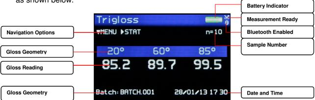
In this mode, measurements can be made by simply pressing the operate button (4) on the instruments keypad.
