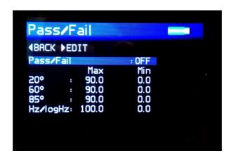
The pass fail set up screen is used to enable/disable on screen pass/fail indication and set measurement criteria.
