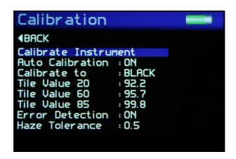
The Calibration Screen is used to setup the instrument calibration to the user's preference. Pressing the Up and Down buttons navigates through the options, pressing the Enter button selects that option.
