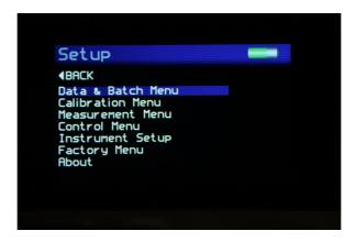
The Setup Screen is used to customise the instrument to the user's preference. Pressing the Up and Down buttons navigates through the options, pressing the Enter button selects that option.
