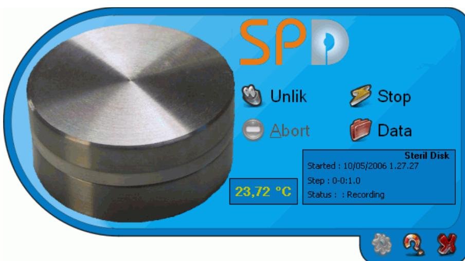
The data acquisition management software for **SterilDisk** is easy to operate, as with all Tecnosoft software programs, but at the same time offers a number of options making it versatile and complete. The program is used to start missions and download data from the dataloggers.
