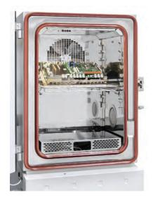
**FLEXIBLE.** As the control and air conditioning compartment are located in the back of the chamber, entry ports are possible from 4 sides: left/right side wall, door, and ceiling. All temperature and humidity chambers feature one 50 mm port on the left and one 125 mm port on the right hand side wall of the test space as standard
