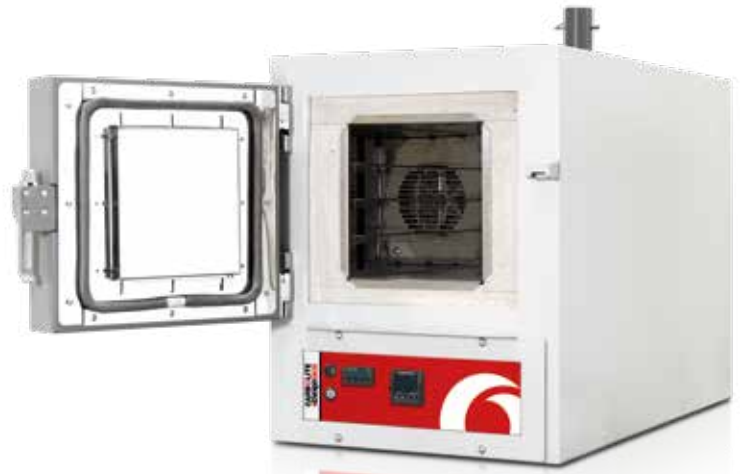
HRF 7/22 with 3216P1 programmer and over-temperature options
