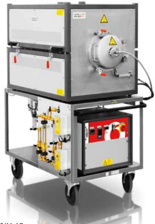
GLO 10/11-1G: Compact hot wall furnace with stainless steel retort and optional inconel retort (vacuum up to 750 °C and under normal pressure up to 1100 °C)
