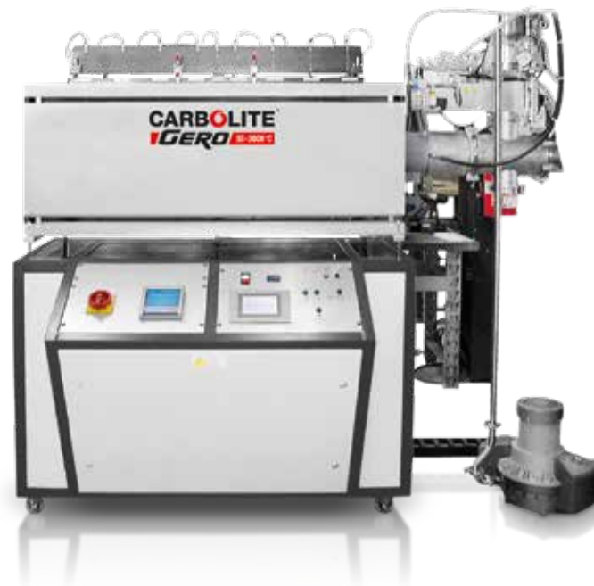
AZ 13/110/1000: This picture shows the high vacuum equipment and touch panel controller option
