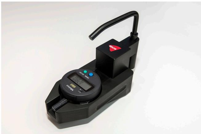
DELTA's Marking Thickness Gauge is a digital device for measuring the thickness of pavement markings dry, after application. The Marking Thickness Gauge is very easy to operate and comes in a sturdy construction and ergonomic design. The Marking Thickness Gauge can measure markings within the measurement range of -12.7 mm to +12.7 mm / -0.5 inch to +0.5 inch. The digital display provides reliable measurement results in seconds.
