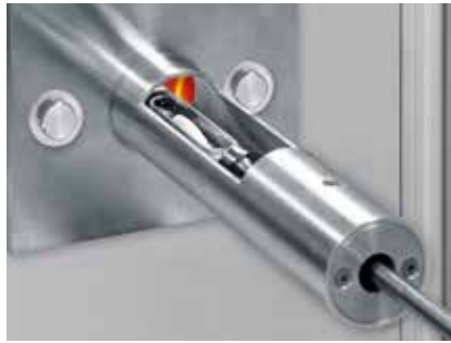
Manual introduction of the sample into the furnace through the loading head
