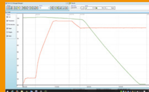
Simultaneous display of temperature (red) and loss in weight (green)
