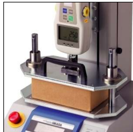
Compression testing on corrugated cardboard
