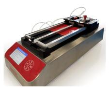
The LR2300 is suitable for a wide range of scrubbing, abrasion and washability tests according to the ASTM, ISO and DIN international standards.
