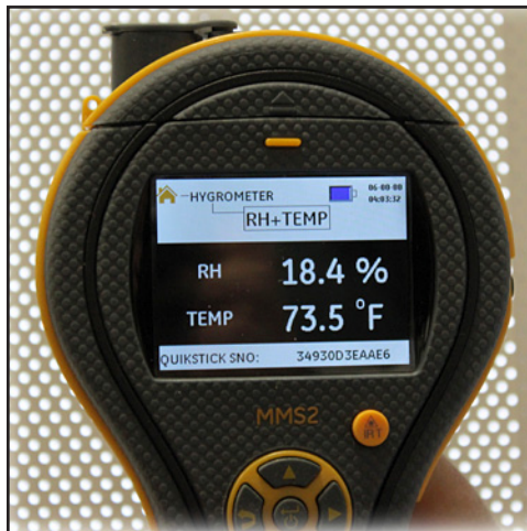
Figure 4: MMS2 as a Hygrometer
