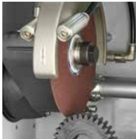
I Large cut-off wheel of 254 mm / 10" with parallel moving wheel guard
