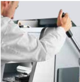
I Manual Y-axis for chop cut with automatic lever brake for easiest handling
