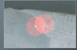
Graphic hint when test points are located to close to each other (3x d) Graphic hint when test points are located to close to each other (3x d)
