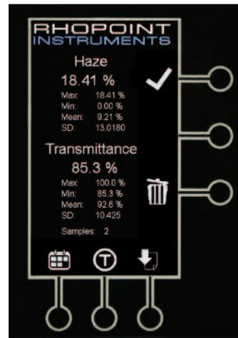
At the end of the test the percentage of Haze and Transmittance are shown on screen.
