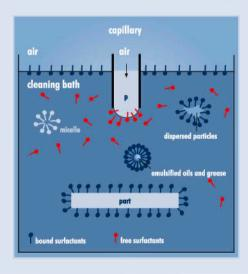
The concentration of free surfactants influencing the cleaning power determines the value of the parameter surface tension.
