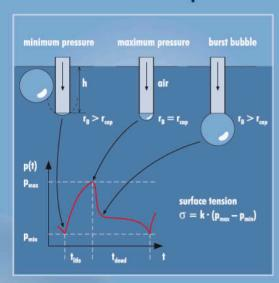
Like all SITA Tensiometers, the SITA clean line ST process measuring device is based on the bubble pressure method to measure the dynamic surface tension in liquids. For this purpose, an air stream is lead into the sample liquid through a capillary which is especially developed for process use.
