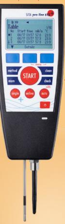
The SITA pro line t15+ efficiently supports analysing surfactant-containing liquids in the laboratory.
