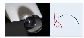
A drop of water is precisely placed at the surface by an automatic dosing unit. The drop is illuminated from the side. A shadow of the drop is projected onto an inclined measuring surface. The projection is recorded from above by a high resolution camera and the picture is corrected for perspective. The drop shape is determined and the contact angle calculated. The lower the contact angle, the higher the wettability.
