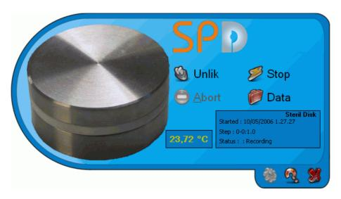
The data acquisition management software for *SterilDisk* is easy to operate, as with all Tecnosoft software programs, but at the same time offers a number of options making it versatile and complete. The program is used to start missions and download data from the dataloggers.
