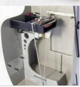
Integrated storage of glass plate and pendulum.
