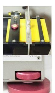
The spirit level is located on the test specimen. Once leveled further calibration is not required.
