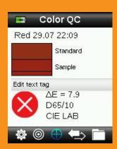
Measure samples and display Pass/Fail warnings. Save up to 350 samples with voice or text tags
