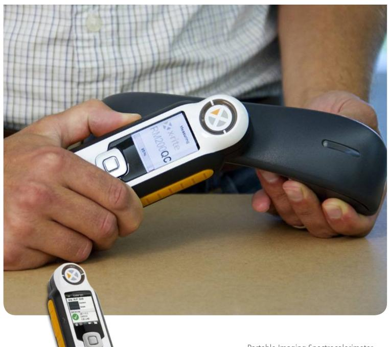
Portable Imaging Spectrocolorimeter
