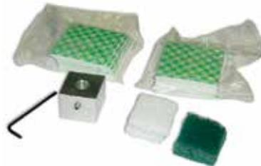
This accessory allows you to simulate the abrasion that occurs when a cleaning or rubbing process is applied to a coating.
