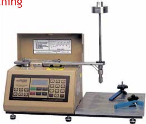
The linear abrasion tester, with adjustable stroke length, speed and load and a wide variety of Wearaser abrasants, enables you to adapt the test parameters to your specific requirements.
