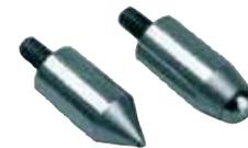
To measure the relative or susceptible resistance of materials to scratching and other similar physical damage. Spherical, semi-spherical, conical and diamond tips available.
