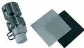
Allows the user to carry out rubbing tests. The commonly used standard abrasants include tools for rubbing fabric or felt. With no extra weight, the base load of the crock test system is: 417.7 + -1 grams, with acrylic finger Ø16 mm.
