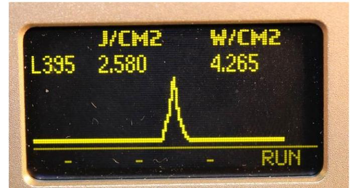
**REFERENCE Mode**– Make a run, data will appear next to the UV band. **CAUTION:** *Be sure you want to overwrite the current data on the REF line before pressing SAVE.* Press **SAVE**, data is transferred to the REF line. The data will remain until it is overwritten.
