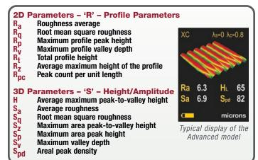
Optical Grade Tape is required for measuring 2D/3D parameters
