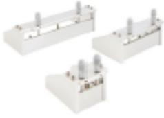
This film applicator includes two integrated micrometric screws to adjust the height of a knife. The distance of this knife can be adjusted in steps of 10 microns from 0 to 6 mm. Produced in hardened stainless steel.
