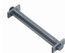
Film applicator of adjustable length. Applicable to thickness in a range of 0 to 250 microns. It can be adjusted making use of the markings on each side of the applicator. Produced in hardened stainless steel.
