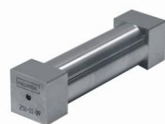
Cylindrical applicator with four defined application heights: 30, 60, 90 y 120 microns or 50,100, 150 y 200 microns. Available in 2 width: 50 and 80 mm.
