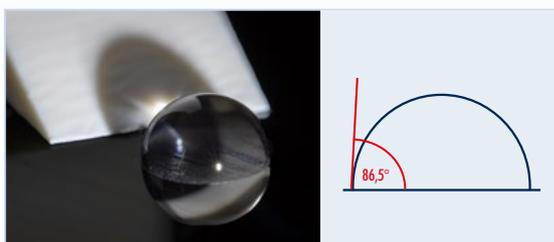
A drop of water is precisely placed at the surface by an automatic dosing unit. The drop is illuminated from the side. A shadow of the drop is projected onto an inclined measuring surface. The projection is recorded from above by a high resolution camera and the picture is corrected for perspective. The drop shape is determined and the contact angle calculated. The lower the contact angle, the higher the wettability.
