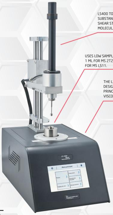
LS400 TOUCH'S SPECIAL FEATURE IS TO STUDY SUBSTANCES AT LOW SHEAR RATES AND LOW SHEAR STRESS, WHICH PREVENTS THE PRODUCT'S MOLECULAR STRUCTURE FROM BEING DAMAGED.
