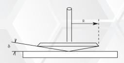
Shear stress / Shear rate  $T = 3M / 2\pi R^3 / D = \omega / arc \delta$
