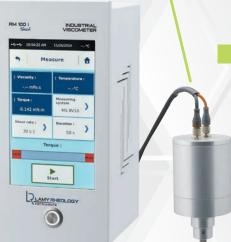
THE DISTANCE BETWEEN MEASURING HEAD AND THE BOX BEING FROM 5 TO 15 METERS, THE RM 100 I TOUCH AND THE RM 100 L TOUCH FIT PERFECTLY TO YOUR VARIOUS LOCATIONS. BOTH INSTRUMENTS HAVE A 4.20 MA ANALOG SIGNAL THAT MEANS YOUR MEASUREMENTS CAN BE CONTINUOUSLY MONITORED.
